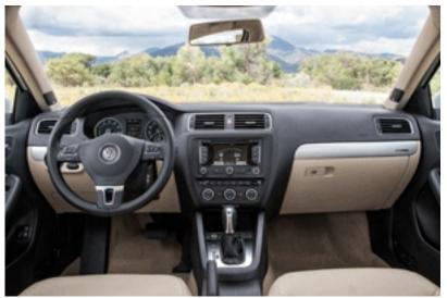
You can monitor your driving efficiency right on the dash. The left gauge in the Hybrid is configured to be a "Power Meter" rather than a tachometer. It starts out at zero, and then goes through a "green regenerator" section, followed by a zero, for when the gauge starts moving. There's a blue section after that showing the best times to be driving, monitoring both gas and
